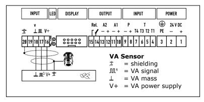
In the case of sensor housings with screwed cable glands, the shielding of the sensor connection cable is connected in the cable glands.
