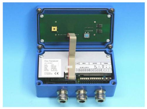
Fig. 2: LCD display connection with cover open
