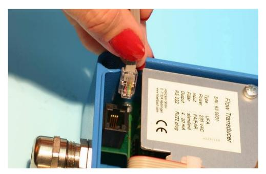
Fig. 1: PC connection with RJ22 plug with cover open
