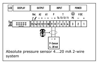
The initial value (4 mA) and the terminal value (20 mA) can be configured with the PC software UCOM VTP via the RS232 interface. Customer-specific programmed values can be found in the accompanying documents.
