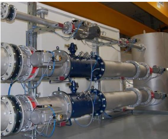
Atmospheric flow rate test bench AVP
