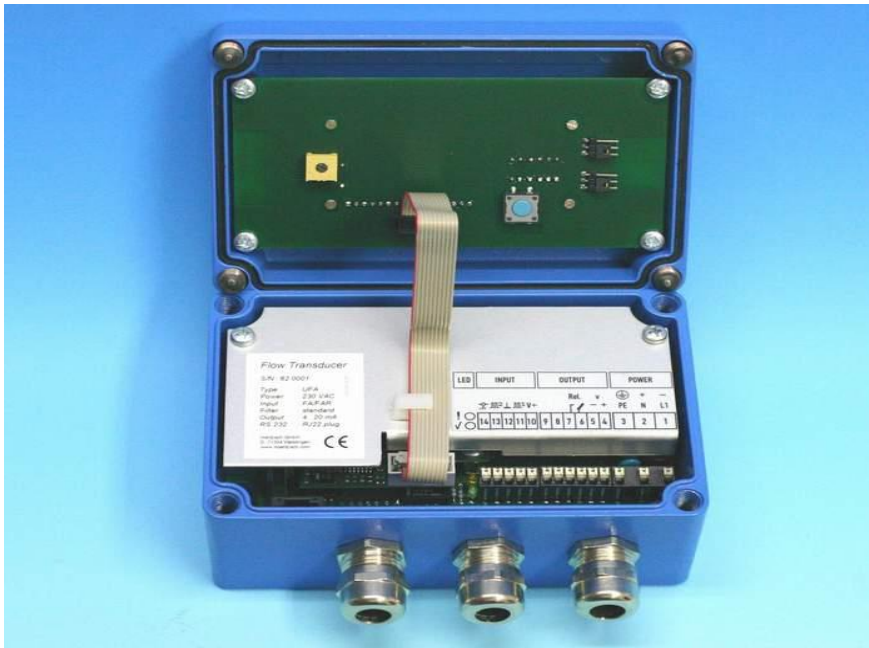
Abb. 2: LCD display connection with cover open
