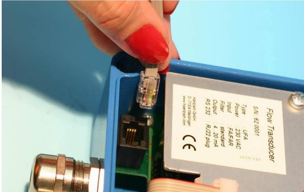
Fig. 1: PC connection with RJ22 plug with cover open
