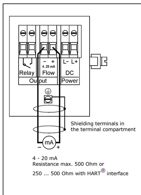
The analog output is configurable with the UCOM software via the HART<sup>®</sup> interface. The factory-set values can be found in the accompanying documents.
