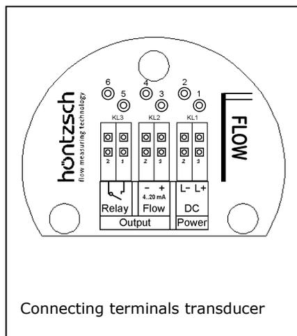
Connecting terminals are accessible after removing the housing cover of the terminal compartment (housing cover on the cable gland side).
