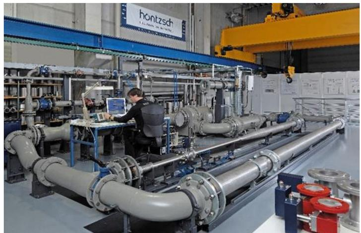
High pressure flow rate test bench HDVP
