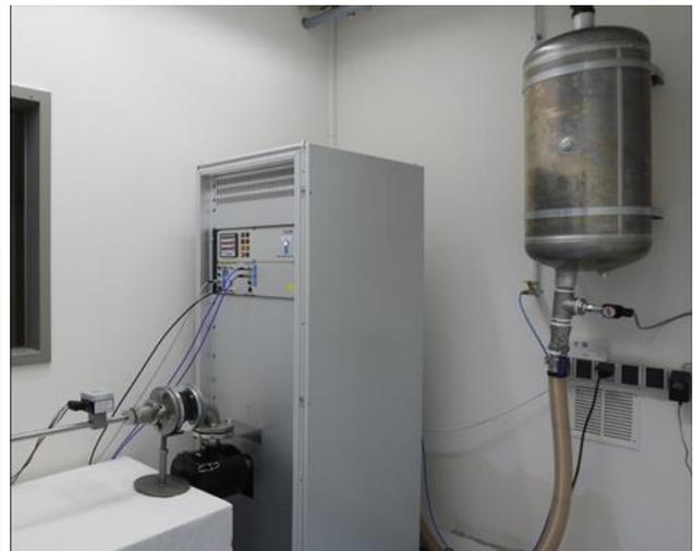
Nozzle flow rate test bench DVP
