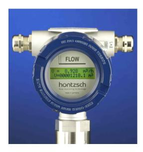
Fig. 1: optional LCD display behind glass
