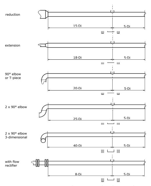
Fig. 3.2-1: necessary input/output sections depending on pipeline positioning
