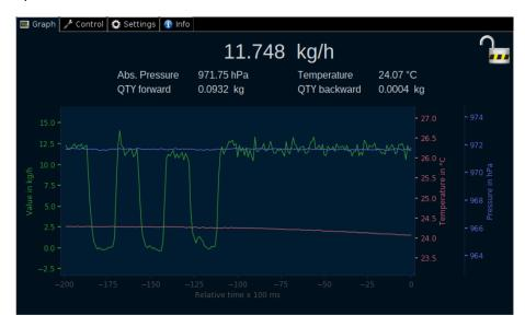
In the Tab Graph, the measured values in the available graphs are displayed averaged over a period of 100 ms. 200 measured values of 100 ms each are shown, which corresponds to an observation period of 20 seconds.
