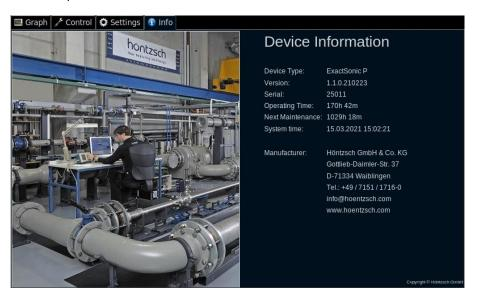
The tab Info contains the device name, the version number, the serial number, the device time and the contact details of Höntzsch GmbH & Co KG.
