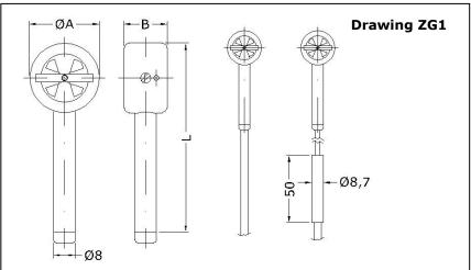
probe line of sight in flow direction, probe sideview, probe without cable amplifier, probe with cable amplifier (in combination with probes for max. +260 °C), from left to right
