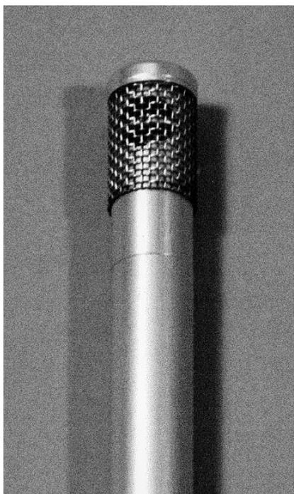
Cylinder probe with protective mesh for measuring water velocity up to max. 1.5 m/s
