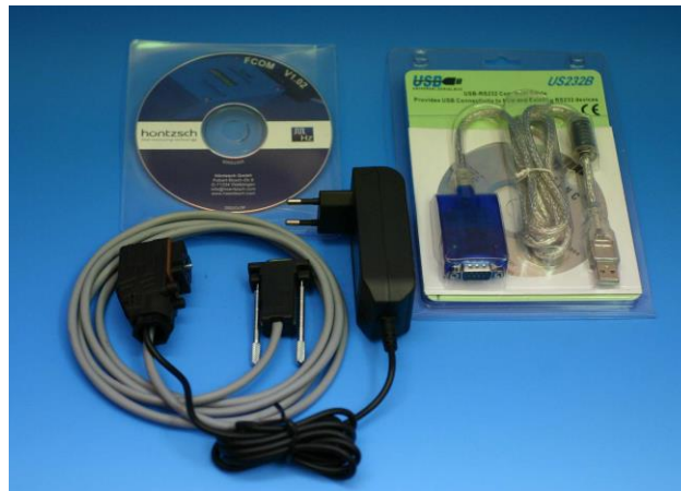
Fig. 1: Programming adapter GO 70 / RS232 for UCOM software, connector PC Sub-D 9-pin, adaptor plug 230 VAC/24VDC and USB adapter
