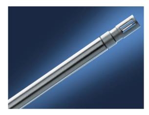
Sensors TA10 / TA Di for explosive atmospheres are simple electrical apparatus for measuring the flow velocity and temperature of air and gases if connected to intrinsically safe apparatus with type of protection **Ex ib.**They are for use in areas in which an explosive gas atmosphere is likely to occur in normal operation occassionally.
