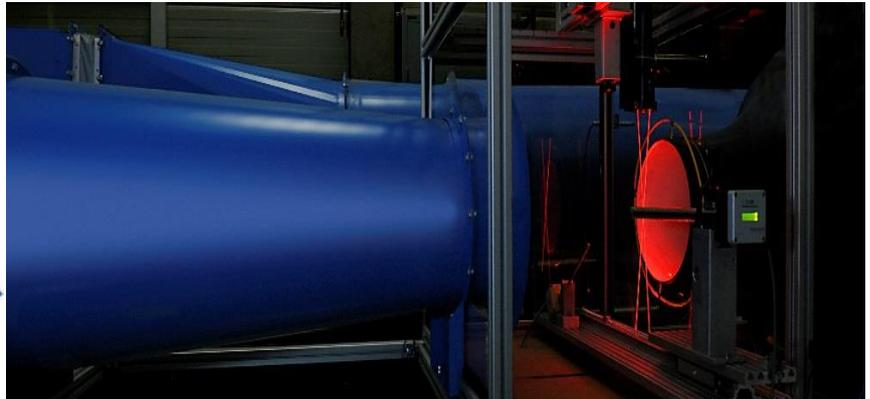
Free jet wind tunnel WK320 with Laser Doppler Anemometer (LDA)
