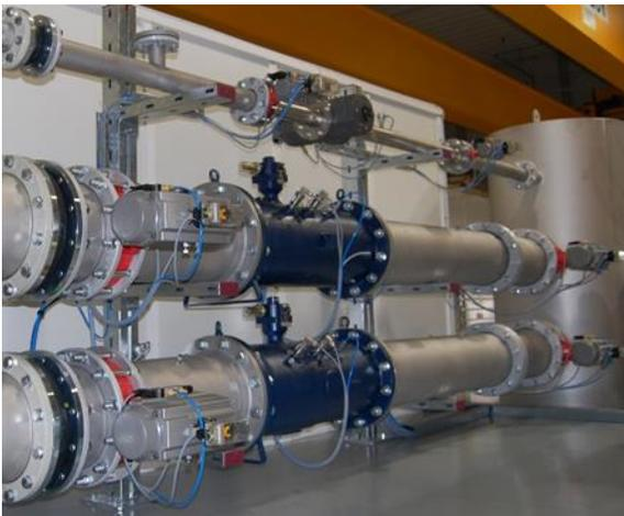
Atmospheric flow rate test bench AVP
