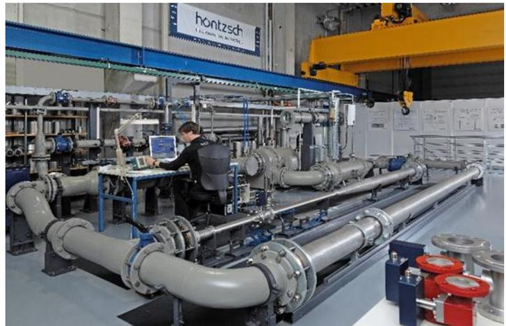
High pressure flow rate test bench HDVP
