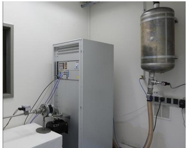
Nozzle flow rate test bench DVP
