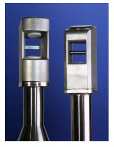
These are intrinsically safe sensors for measuring the flow velocity of gases and designed for use in areas in which an explosive gas atmosphere is likely to occur in normal operation occasionally.
