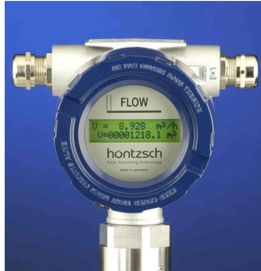
Fig. 1: optional LCD display behind glass
