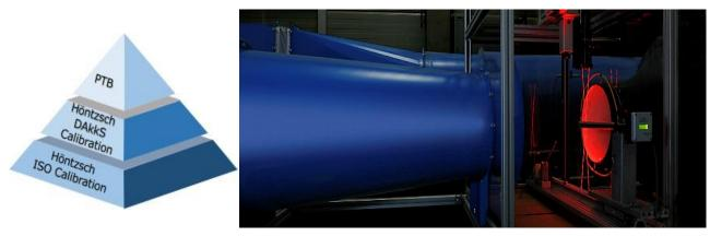
Free jet wind tunnel WK320 with Laser Doppler Anemometer (LDA)
