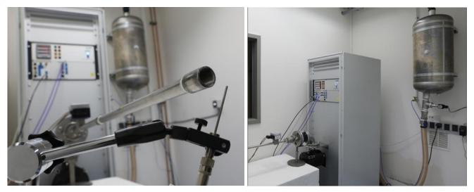
Nozzle flow rate test bench DVP
