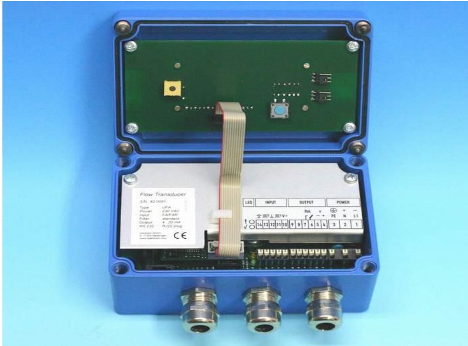
Fig. 2: LCD display connection with cover open
