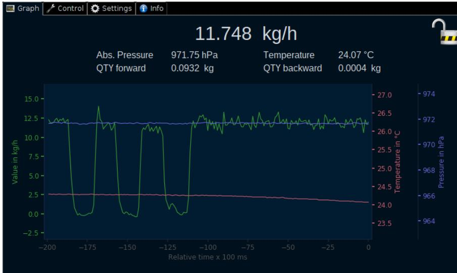
In the Tab Graph, the measured values in the available graphs are displayed averaged over a period of 100 ms. 200 measured values of 100 ms each are shown, which corresponds to an observation period of 20 seconds.
