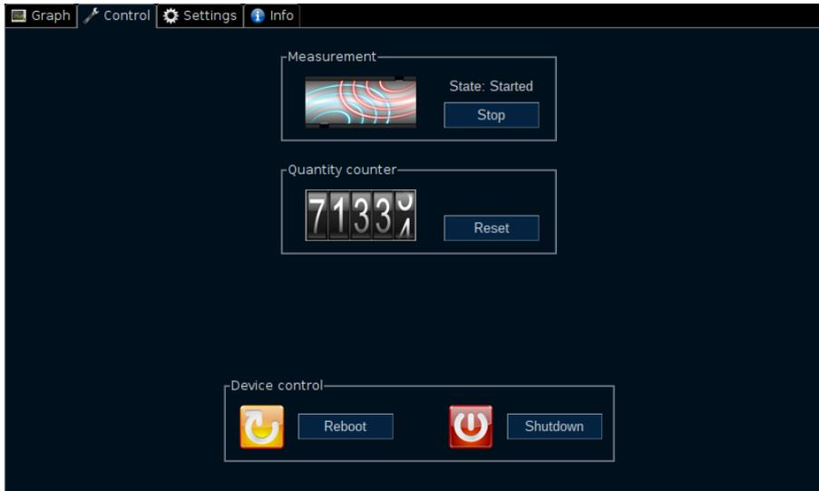
In Tab Control the measurement can be paused. The graph is no longer updated when the measurement function is stopped; the last measured value is permanently displayed. The measurement data via TCP interface also no longer change, the last measured values are always transmitted. The analog output is also frozen at the last value.
