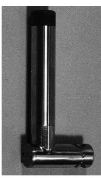
Cylinder probe with 90° elbow
