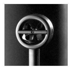
T-probe withvery small size, 16 mm long, shaft diameter 8 mm, sensing ±direction of flow
