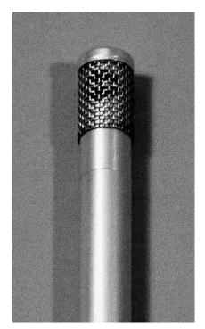
Cylinder probe with protective mesh for measuring water velocity up to max. 1.5 m/s
