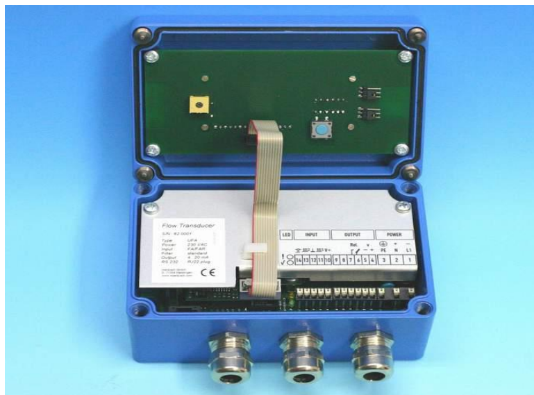
Fig. 2: LCD display connection with cover open
